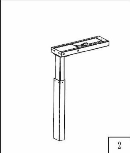
2. Install the top support with Allen key ( Pic 3 and Pic 4 )
